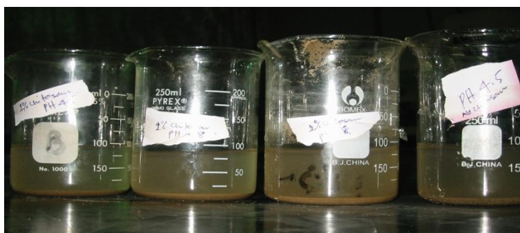
Fig.-7: Experimental work on Chitosan Dosage against variable pH values
